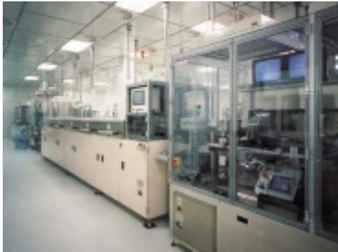
Fig. 18: Display Fabrication has to be carried out in clean room environment. (Picture courtesy of Optrex Europe)
