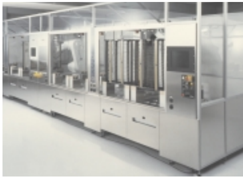
Automation system for New Aristo sputtering machine
