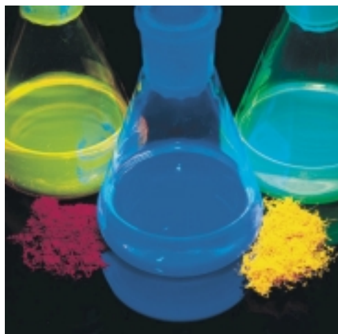
Fig. 21: The basic materials for OLED displays: Small molecule and polymer OLEDs. (Picture courtesy of Covion)
