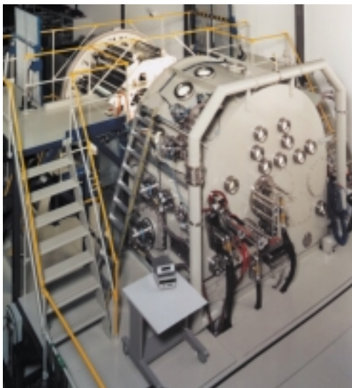
Fig. 22: Potential low-cost OLED fabrication with reel-to-reel process. (Picture courtesy of Fraunhofer Institut FEP)
