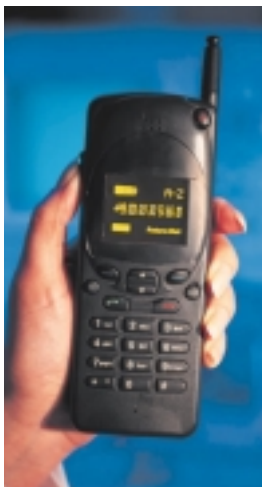
Fig. 14: One of the first products where OLED display will be commercially available. (Picture courtesy of Covion)
