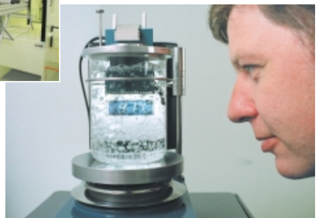
LCD with enlarged T-range with colorPol® polariser
